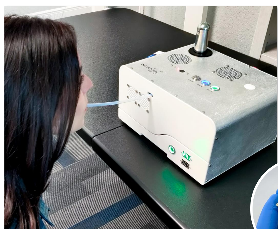
Point-of-Care CLARION Breath Diagnostics (Top) powered by Detect-ION's chip-scale mass spectrometry (Right) enables real-time breath analysis for rapid detection of infectious diseases.
