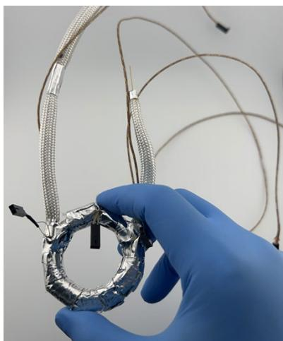
**Figure 2.** A prototype of the 10-m LTM-GC that delivers high-speed gas chromatography needed to separate individual constituent chemicals from a complex chemical mixture before delivering the gas bolus to the  $\mu$ MS for chemical detection.
