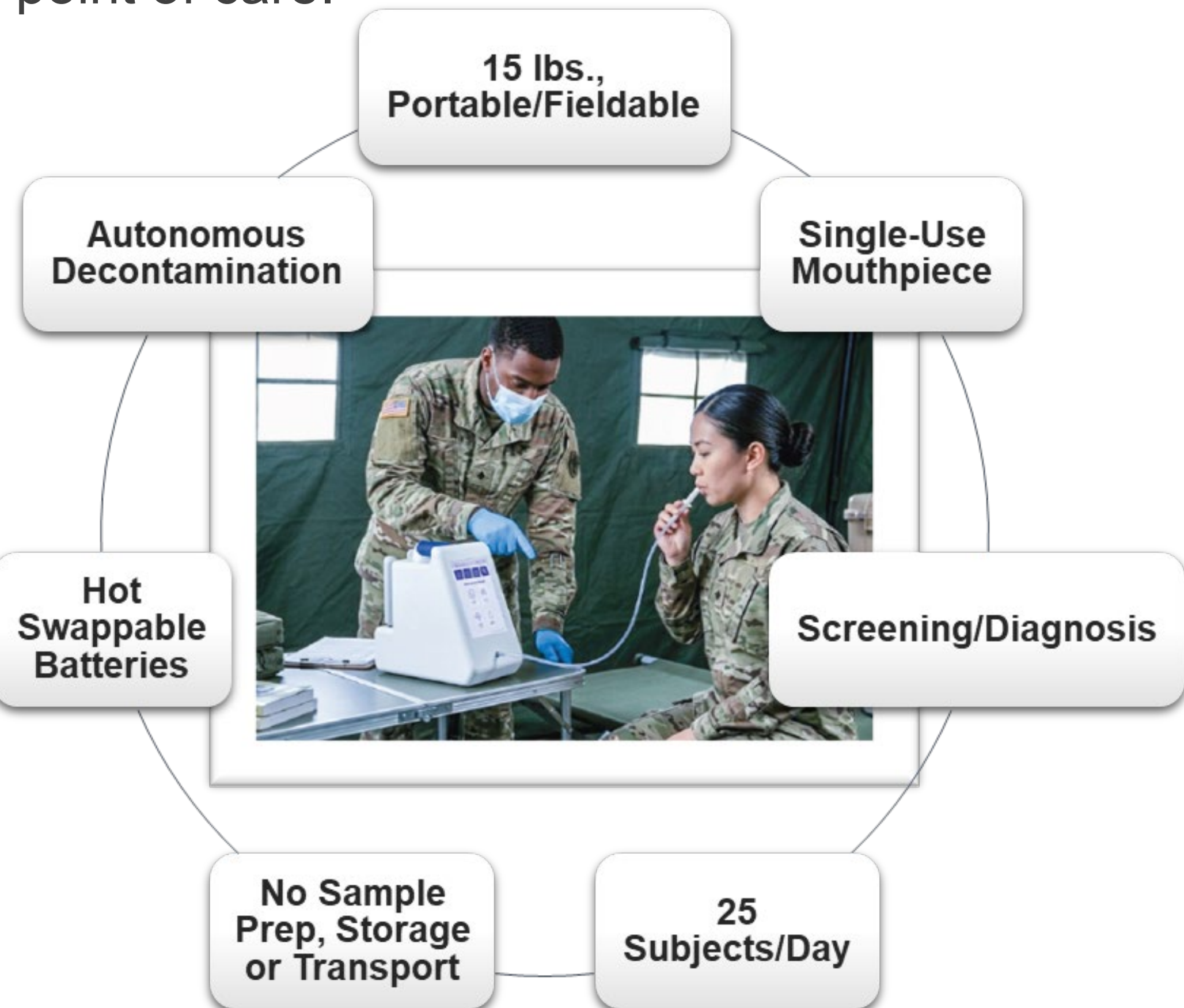
Figure 1. CLARION collects and analyzes exhaled human breath in a field-forward austere environment thereby enabling laboratory-grade GC-MS analytical capability in a decentralized outdoor setting.
