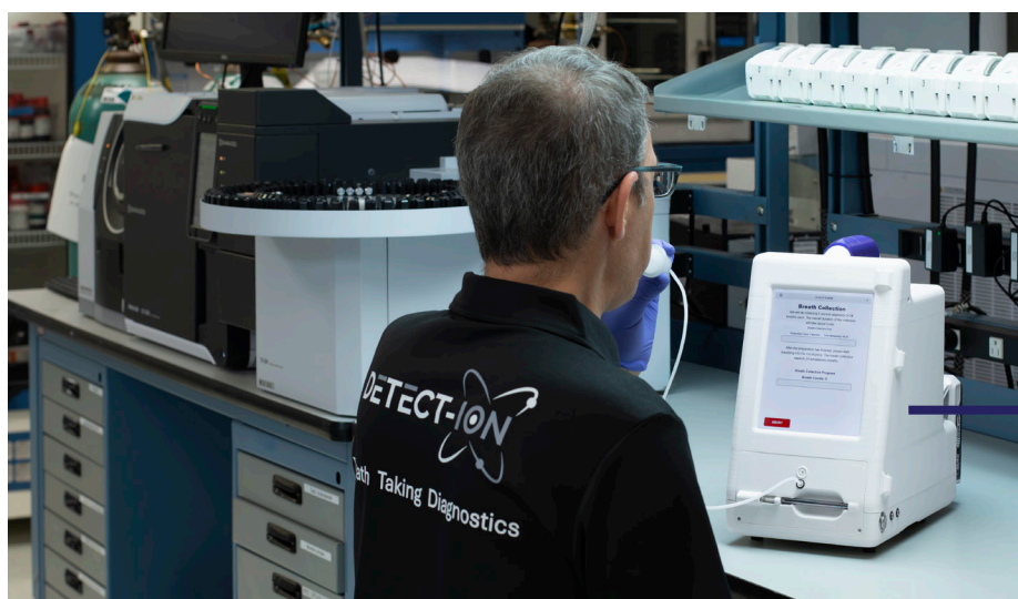
Figure 3. Left: In the background, a laboratory-bound Shimadzu TD-GC-MS traditionally used for breath analysis. Right: A subject breathing into the Point of Care Breath Diagnostic Platform (CLARION-β) for real-time health assessment.
