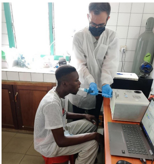
Figure 4. A subject in Brazzaville exhaling into the CLARION-α system to provide a specimen for subsequent breath analysis during HT-1.
